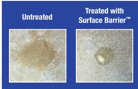
The stone surfaces above were affected by mineral seal oil. On the left (untreated side), the oil has left an immediate stain, while the oil on the right side (treated with Surface Barrier™) has "beaded-up" and can be removed easily without staining the stone.
